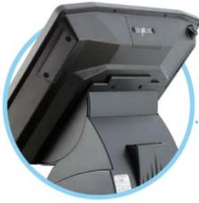
**Aluminium Die-cast Casing**
